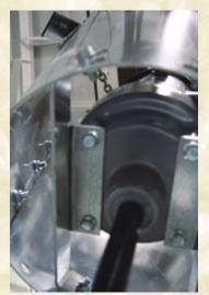
Totally-enclosed C-face motor is mounted directly to an in-line gear reducer for no loss of horsepower and no belts to maintain or replace.
