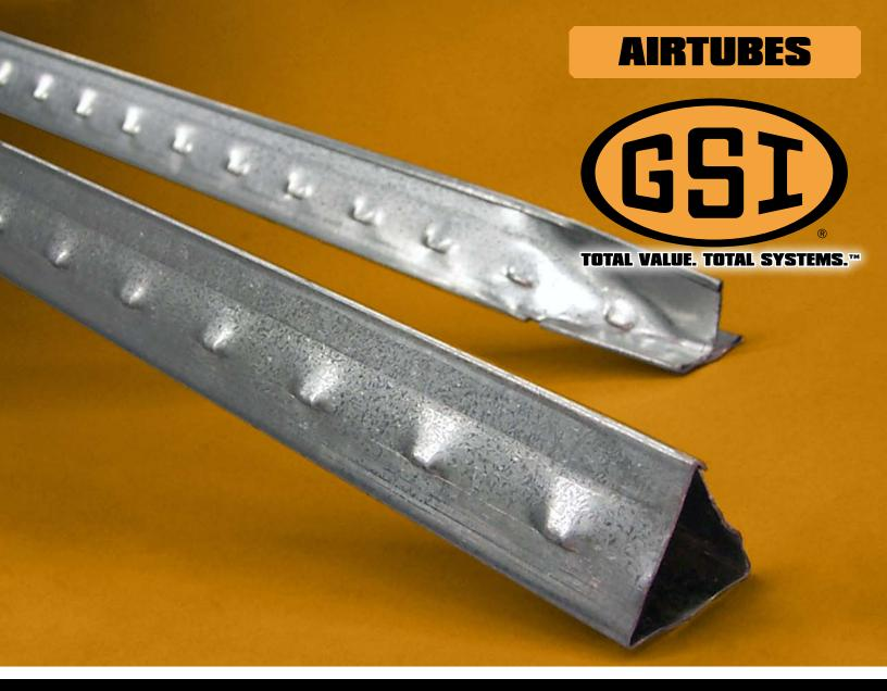
GSI's AirTubes are triangular aeration pipes attached vertically to the inside of the bin sidewall. AirTubes prevent sidewall moisture condensation and freezing which can cause extensive grain spoilage and bin damage. Other benefits include reduced drying times due to wider aeration coverage and simple installation.
