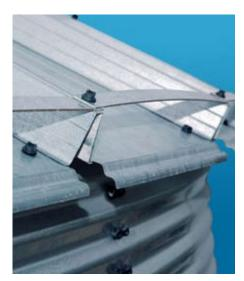
**"High-rise" roof rib** is a full 3 inches (76 mm) tall and utilizes Brock's strengthgiving 2-step rib design. Brock's innovative **Eave Tension Straps** offer the highest farm bin peak load capacities available, up to 8,000 pounds (3,600 kg) with a ground snow load rating of 30 pounds per square foot (146 kg per square meter).
