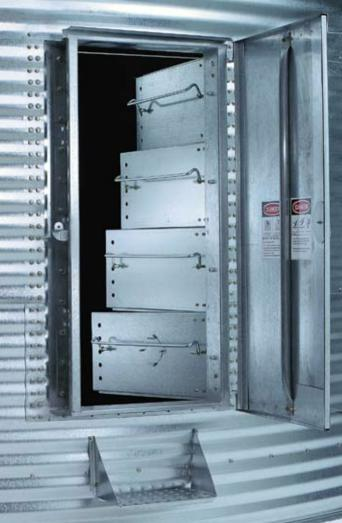
Industry-leading bin accessories like Brock's LATCH-LOCK<sup>®</sup> Walk-Through Bin Door make grain storage manageable with the least amount of hassle. The one-piece outer door opens wide to fasten securely against the side of the bin. The four interlocking inner panels open in sequence from top to bottom with a simple lift of the patented latches. No tools required.
