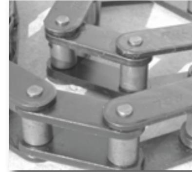
The steel chain is 81x and 81xH 24,000 and 44,000 lb. average ultimate strength. Welded channel attachments add rigid support for paddles. In larger capacity or long conveyors dual chains are used. Paddles are 1/2" thick UHMW CNC manufactured for accuracy. UHMW prevents metal to metal contact reducing HP requirements and increasing conveyor life.
