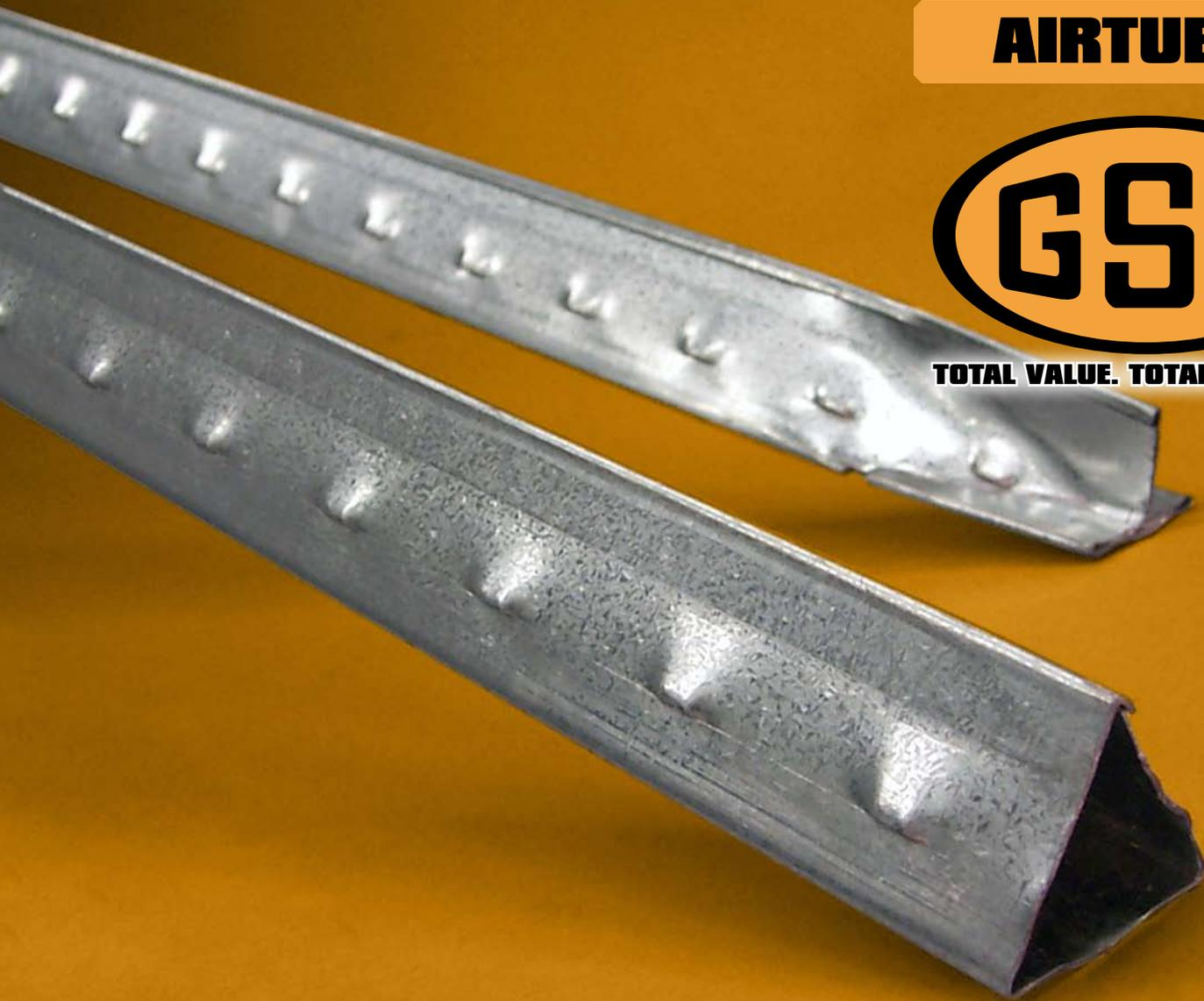
GSI's AirTubes are triangular aeration pipes attached vertically to the inside of the bin sidewall. AirTubes prevent sidewall moisture condensation and freezing which can cause extensive grain spoilage and bin damage. Other benefits include reduced drying times due to wider aeration coverage and simple installation.
