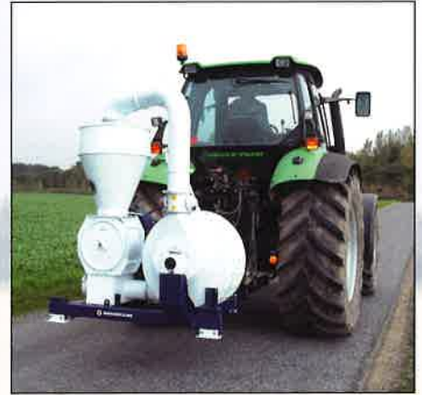
Tractor powered Grain Vacs type SUC-T mounted on the lift arm and driven by the PTO shaft. Available in 2 sizes with a capacity of up to 1,800 bushels (33 tons)/hour.
