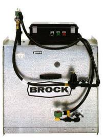
**Heater models** are available for use with liquid propane, propane vapor, or natural gas fuels and utilize gas-certified solenoid valves. Brock-supplied regulators are standard on liquid propane models.
