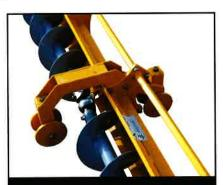
Pre-Set Carrier Wheels enable steady movement of the sweep across the floor. Eliminates the need for bin entry and set-up prior to sweep activation.
