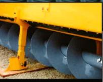
Innovative Flighting has thicker outer edge to increase auger capacity up to 100 bushels (2.5 metric tons) per hour and to extend the auger's lifespan.
